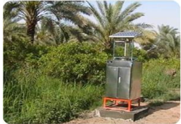
Figure 1. Light traps that were used to collect borers' adults from date palm trees Phoenix dactylifera L.
