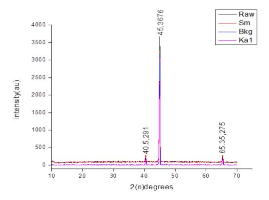
Figure 2. XRD pattern showing peaks at 40.0°, 44.7° and 65.9°.
