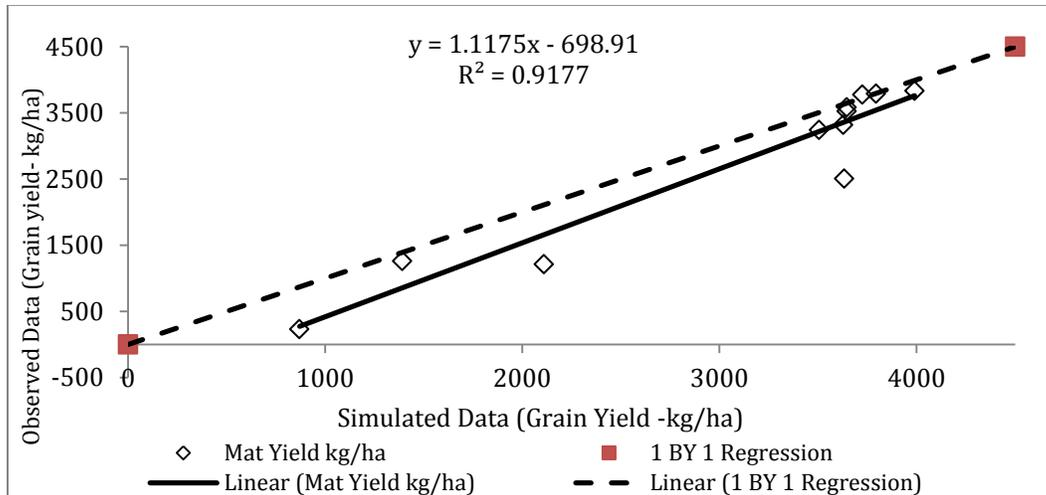
Figure 1. Comparison of grain yield predicted by the DSSAT model with measured values.
