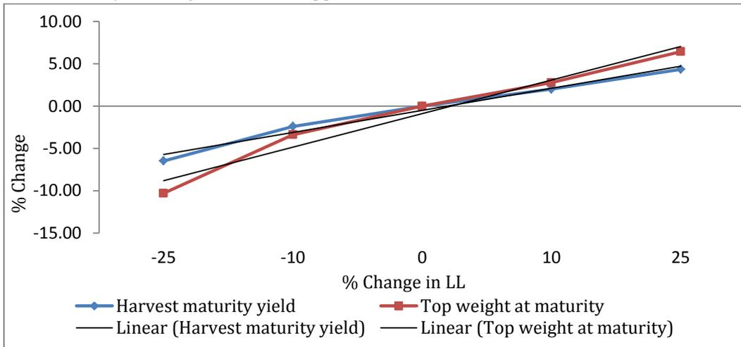
Figure 6b. Model sensitivity to changes in lower limit of available soil water
