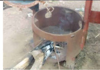
Figure 2. Improved hearth directly integrated to the improved 180 kg device (Kpossilandé, 2022)
