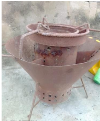
Figure 10. Improved rice husk metal hearth (Kpossilandé, 2022)
