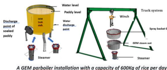
Figure 4. A GEM parboiler with a capacity of 600 kg of rice per day (TAAT, 2021)
